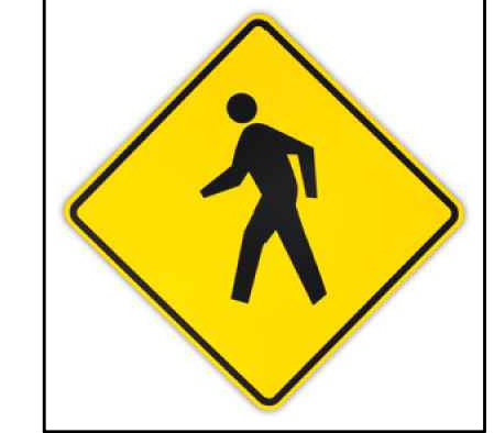
SIGN DETAIL W11-2 DETAIL (30" x 30")
