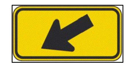
SIGN DETAIL W16-7p DETAIL (30" x 18")
